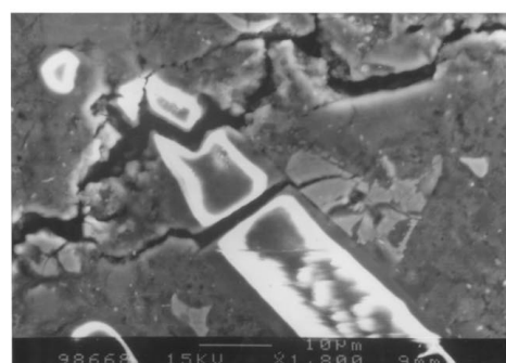
Figure 3 SEM micrograph of thermal fatigue crack morphology. (a) AlSi12CuMgNi; (b) 18%Al 2 O 3sf /AlSi12CuMgNi.
